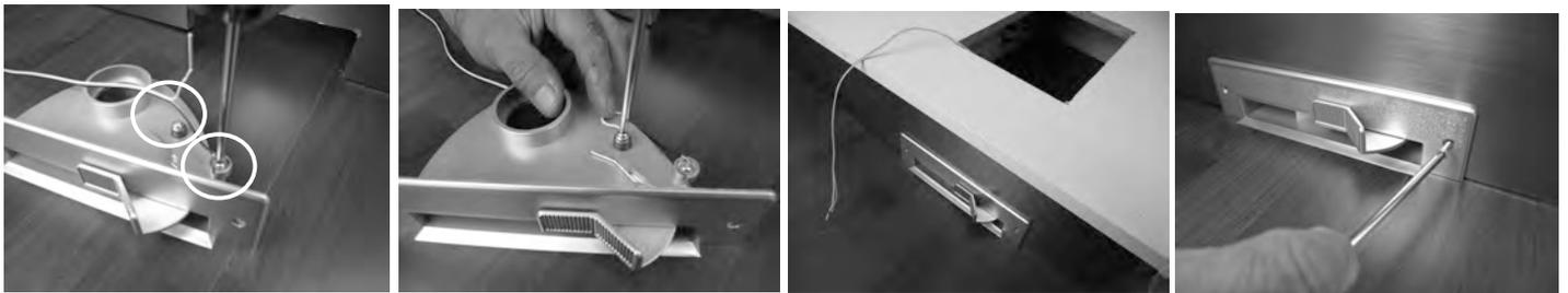
Connect the Figure 8 cable to the dustpan inlet. Attach wires on each screw as shown, polarity does not matter. Then fit dustpan inlet into cutout in the kickboard, with the cable inside the cavity and feeding it through the main rectangle you cut out as shown. Finally, secure dustpan inlet with the 2 screws to the fascia of the kickboard.
