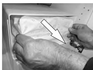
3. Remove Adaptor port from Filter bag and dispose Filter bag.
