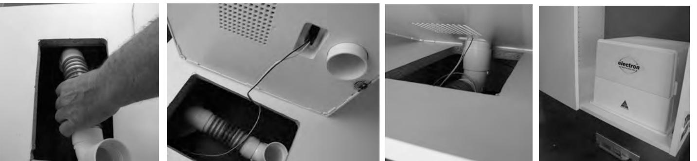
Connect the figure 8 cable to the terminals of the vacuum unit. One wire on black and the other on red terminal. Connect one end of the pipe manifold to the dustpan inlet and the other end to the vacuum unit. Do not glue. Once cable and pipe manifold are connected, place vacuum unit on the board surface and secure with 4 screws. Connect power cord to vacuum unit and then to the power point. Your Electron built in mini vac is now ready to use. Congratulations!
